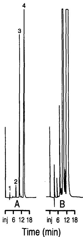
Fig. 1. Separation of SFO-LSO methyl ester standard. Flow-rate: 1.0 ml/min 0.2% ACN in hexane. UV detection at 210 nm. Sample size: A = 17 \mu g; B = 170 \mu g. Peaks: 1 = 16:0 and 18:0; 2 = 18:1; 3 = 18:2; 4 = 18:3.
